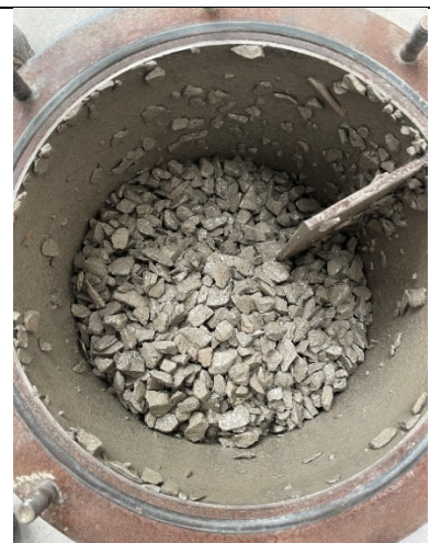
Figure 3 : Aggregate coated with pre-dispersed NGDA
