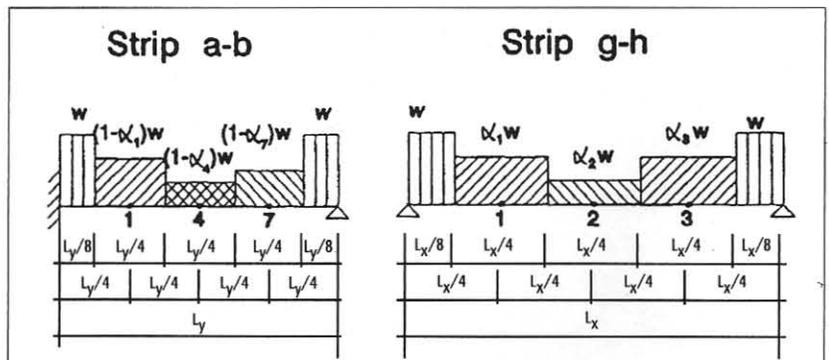
Figure 4 - Example of division of load onto orthogonal strips
