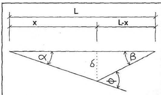
Figure 7 - Calculation of deflection due to hinge at crack
