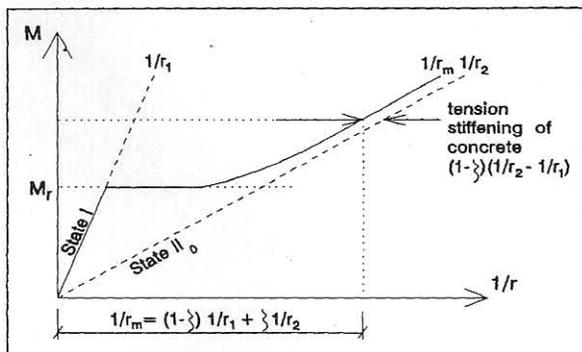
Figure 1 - Instantaneous moment - curvature relationship after Manual on CEB/FIP Model Code (2)
