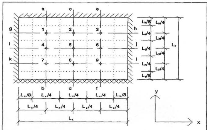
Figure 3 - Division of slab into strips (between dotted lines)
