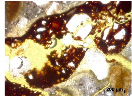
Microscopic image of horizontal crack filled with corrosion particles
