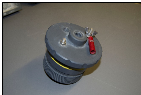
Figure 4.3: Connecting point of chloride conductivity cell
