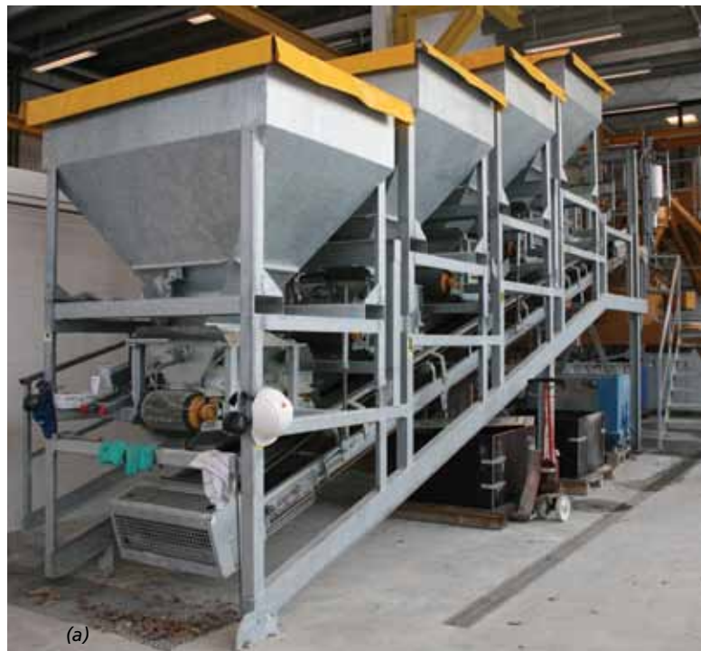
Fig. 2: High-Technology Concrete Laboratory at DTI: (a) automatic concrete batch plant; and (b) industrial robot
