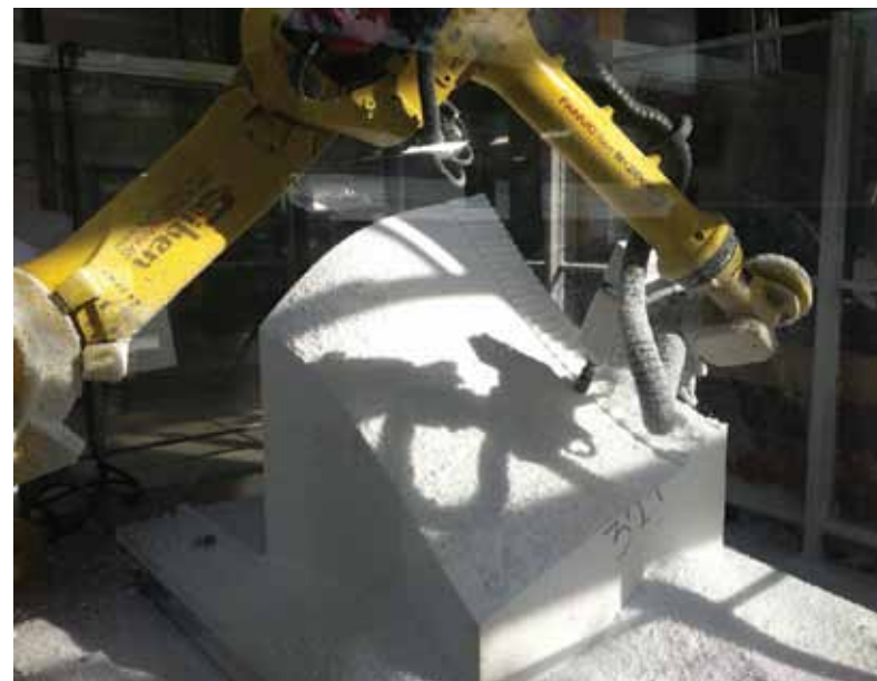
Fig. 4: Manufacturing of formwork blocks using five-axis milling at DTI
