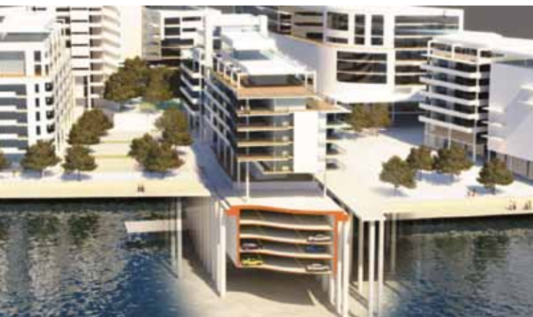
Fig. 2: Large, prefabricated concrete caissons shown in rendering provide up to four levels of submerged parking.
