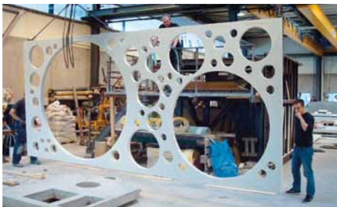
Façade element produced in light CRC at Hi-Con
