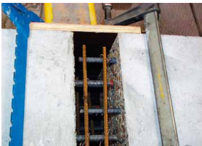
Joint between two concrete beams with 80 mm lap between 12 mm diameter bars
