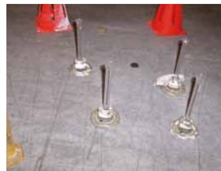
Figure 2: Testing for relative absorption using Rilem tubes. In this case, four tubes were used at each test site/cycle.
