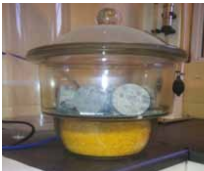
Figure 2.3: Cored Discs Samples Stored in a Desiccator
