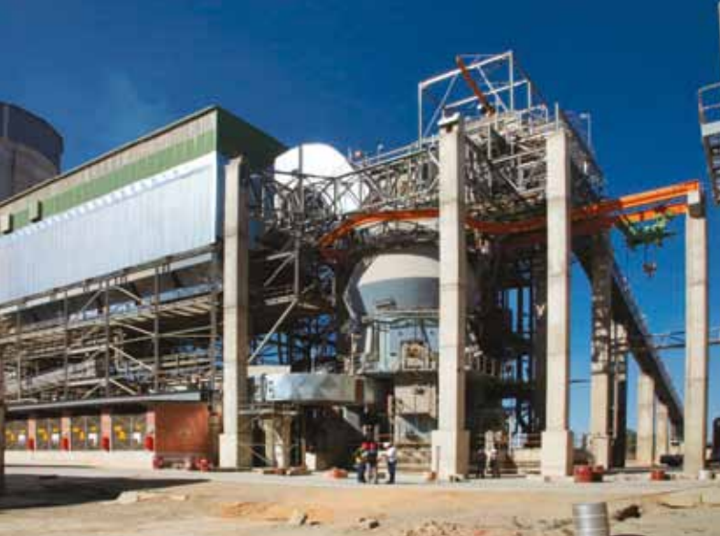
The vertical roller mill at AfriSam's Roodepoort cement operation has contributed to a 20% reduction in energy consumption since its installation in 2008.
