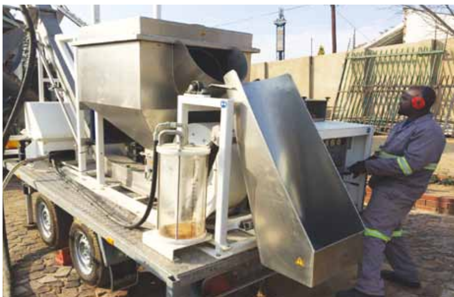
Special machine for blowing and dispensing steel fibres into the mixer
