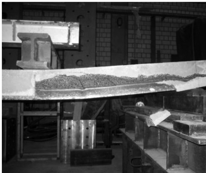
Figure 7. Specimen A at the ultimate limit state.
