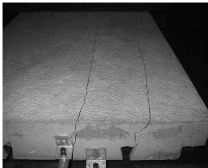
Figure 9. Longitudinal splitting cracks in specimen A.
