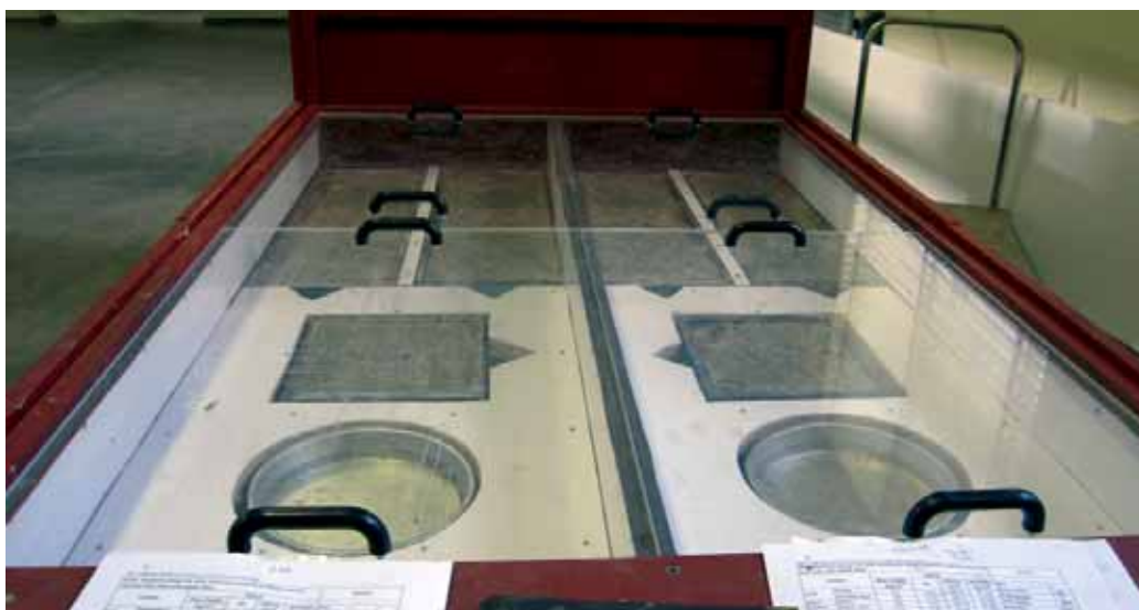
Figure 3: Climate chamber for the testing of plastic shrinkage cracking.
