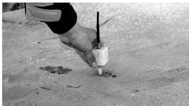
Figure 4: Wireless capillary pressure sensor to be used for on-site measurements.
