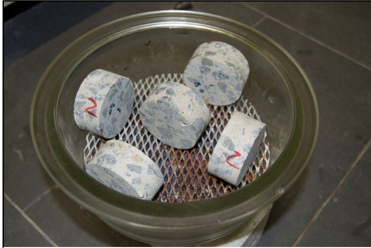
Figure 3.5: Illustration of recommended arrangement of specimens for saturation
