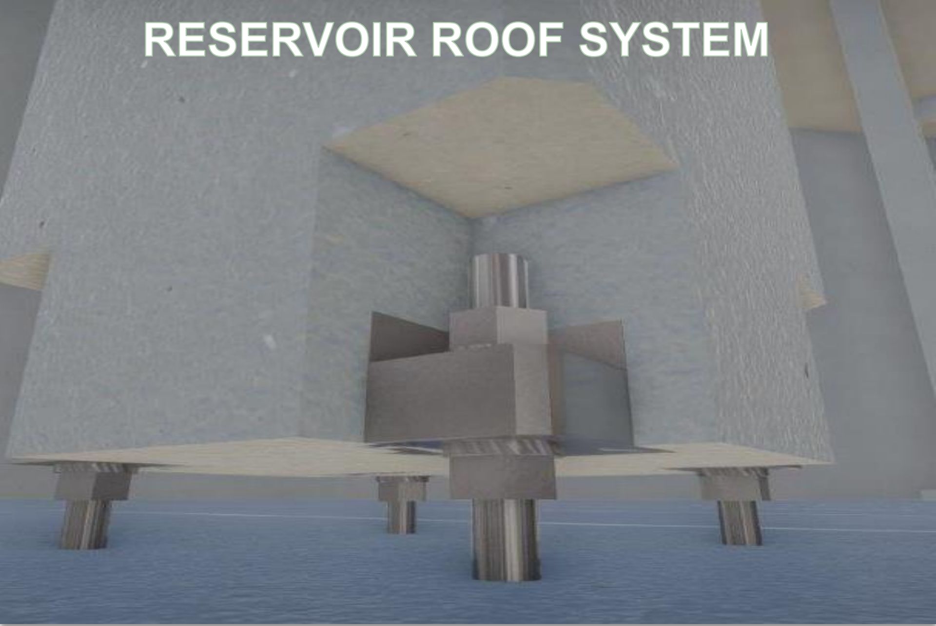
Typical Column to Base/Footing connection
